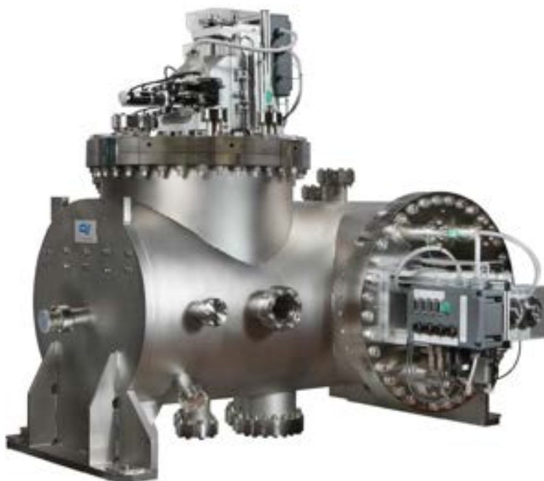
Figure 9.11: An example of commercial K-B system: the KAOS system developed at Elettra (from [14]).
