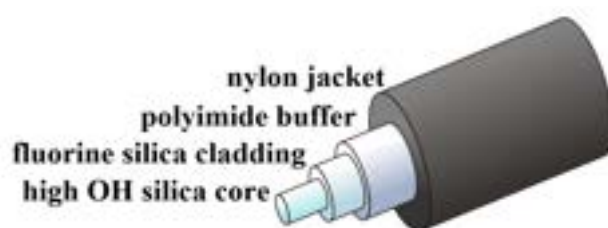
Figure 11.27: Internal structure of high-OH silica core fiber.
