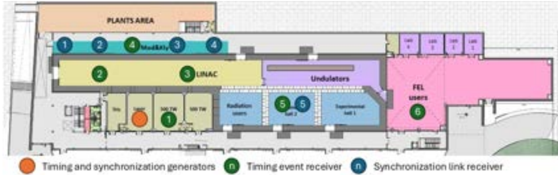
Figure 14.1: Map of the Timing and synchronization hardware on the level L0 building plan.
