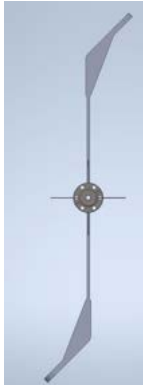
Figure 8.52: Front view of the undulator vacuum chamber. The holders to be fixed to the undulator frame are visible in the upper and lower side of the chamber axis.
