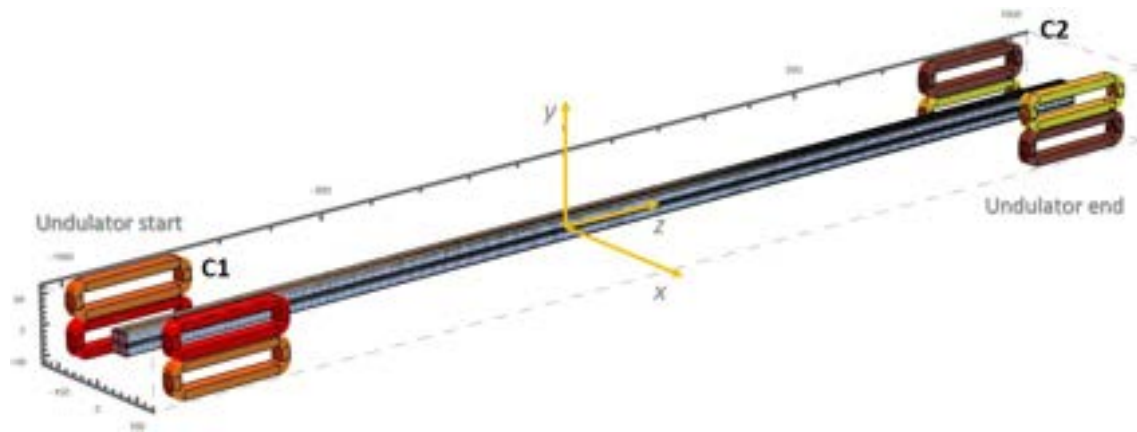
Figure 8.24: Correction coils scheme and its displacement at the begin (C1) and at the end (C2) of the undulator magnets array. Coils with the same color are electrically coupled in series.
