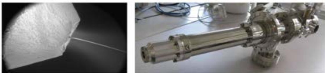
Figure 10.2: An overview of sample injection systems that will be installed at AQUA. An environmental scanning electron microscope picture of a GVDN producing a micrometer-sized water jet (left panel). A stack of aerodynamic lenses used for aerosol injection (right panel).
