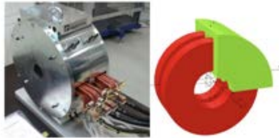
Figure 17.1: SPARC_LAB gun solenoid and its 3D model
