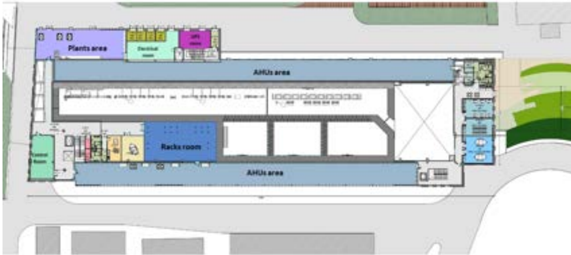
Figure 18.8: EuPRAXIA@SPARC_LAB building functional layout - Level 1.
