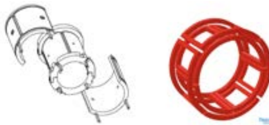
Figure 17.3: Design of the skew quadrupole mounted in the gun solenoid
