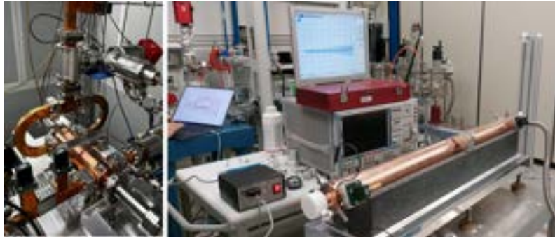
Figure 6.11: X-band accelerating structure prototypes: 20 cell structure under high power testing at the LNF TEX test facility (left); full scale rf structure under low power rf characterization (right).
